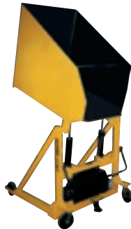
PORTABLE DUMPER W/ NARROW DISCHARGE CHUTE
